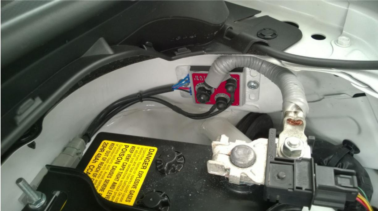
The Isolator should be mounted directly to the vehicle's metal chassis close to the vehicle's battery but away from any high temperature sources.
