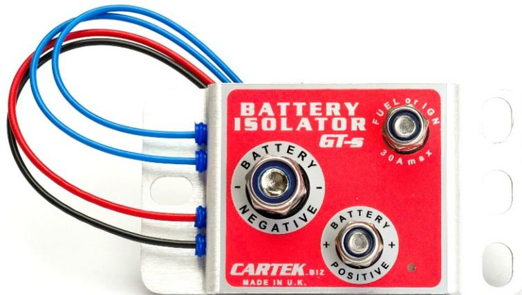
The **CARTEK Battery Isolator GT** is a fully electronic 'master/kill switch' system designed specifically for race car applications. This device contains no moving parts and the solid construction provides very high resistance to shock, vibration, water and dirt. Using the latest MOSFET technology this Battery Isolator provides safe, spark-free isolation of the vehicle's battery and engine electrics.
